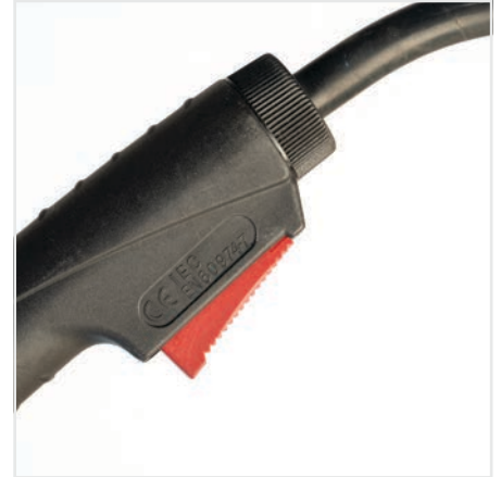
(8) Press and hold the Torch Trigger to feed the wire down the torch cable through to the torch head.
