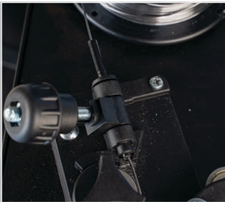
(4) Snip the wire carefully, be sure to hold the wire to prevent the spool uncoiling. Carefully feed the wire into the inlet guide tube of the wire feed unit.
