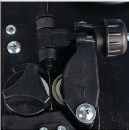
(7) Close down the top roller bracket and clip the pressure arm into place. Apply a medium amount of pressure to the drive roller
