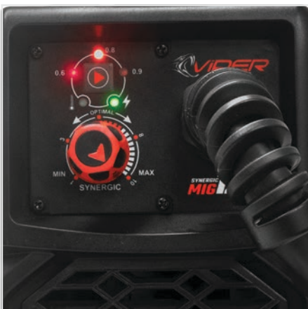
(13) Select wire size, then adjust synergic control knob to suit work piece.
