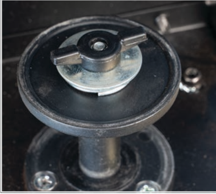
(1) Remove the spool retaining nut.
