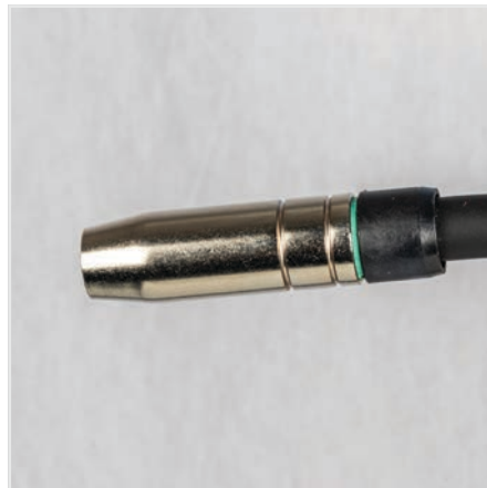
(11) Fit the gas nozzle to the torch head.
