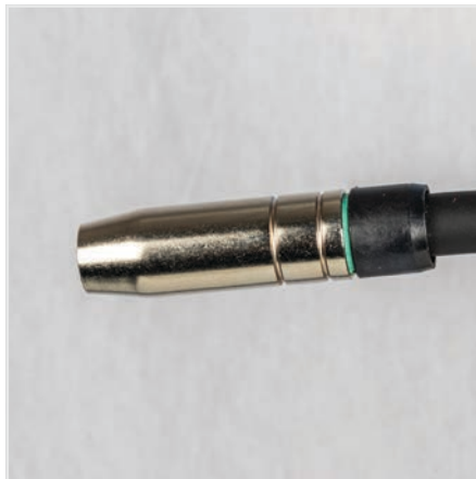
(10) Fit the gas nozzle to the torch head.
