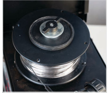
(3) Fit the wire spool onto the spool holder fitting the locating pin into the location hole on the spool. Replace the spool retaining nut tightly
