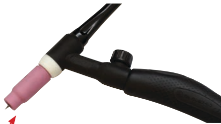
(5) Assemble front end parts of the TIG torch, fitting a sharpened tungsten suitable for DC welding.
