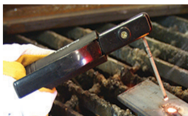
(7) To finish the weld, break the arc by quickly snapping the electrode away from the work piece.
