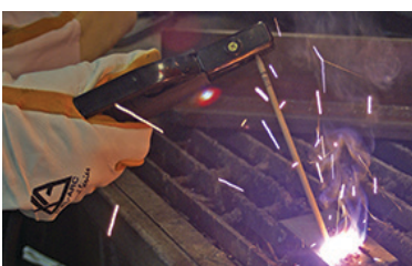
(6) Hold the electrode slightly above the work maintaining the arc while travelling at an even speed.
