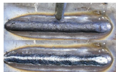
(8) Wait for the weld to cool and carefully chip away the slag to reveal the weld metal below.
