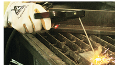
(5) Strike the electrode against the work piece to create and arc and hold the electrode steady to maintain the arc
